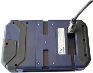
Fig. 10: Camera cable connection
