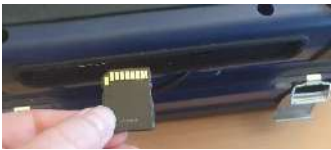
Fig. 9: Insert SD card correctly
