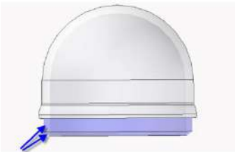
Fig. 68: Fitting the camera dome
