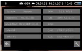
Fig. 52: Info menu with SOM (Firmware of the camera) and CAM (Version of the camera head)
