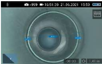
Fig. 43: Distance between 2 measuring points
