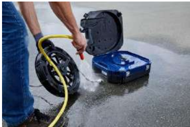
Fig. 77: Cleaning the viper and the rod
