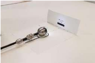
Fig. 47: Calibration with calibration template
