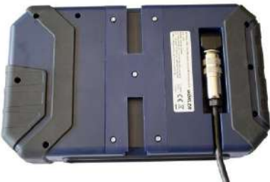
Fig. 11: Camera cable fed through guide
