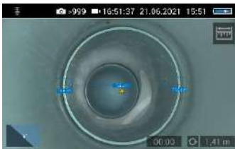
Fig. 44: Warning triangle under distance indicator
