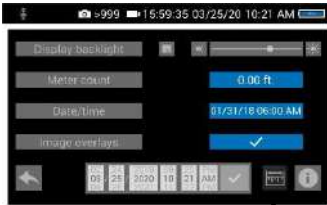
Fig. 48: Icon „distance measurement“ in the settings menu
