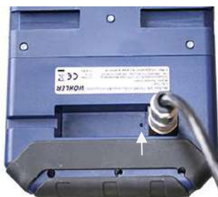
Fig. 67: Reset hole indicated by an arrow
