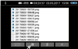
Fig. 37: Image gallery with highlighted files; the Save icon is indicated by an arrow.
