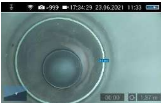
Fig. 26: Focus adjustment , distance is displayed
