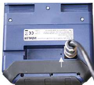
Fig. 69: Reset hole indicated by an arrow
