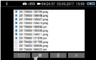
Fig. 39: Image gallery with highlighted files; the Save icon is indicated by an arrow.
