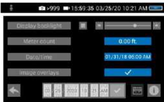
Fig. 48: Settings menu, menu point „Image overlays“ is activated
