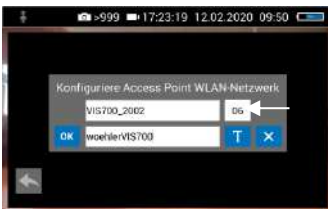
Fig. 61: WLAN-channel marked by arrow
