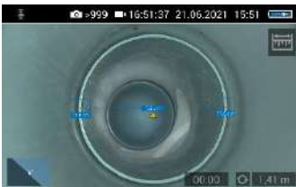
Fig. 46: Warning triangle under distance indicator
