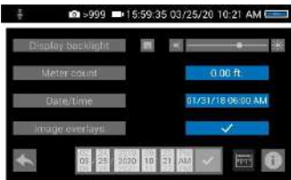
Fig. 46: Settings menu, menu point „Image overlays“ is activated
