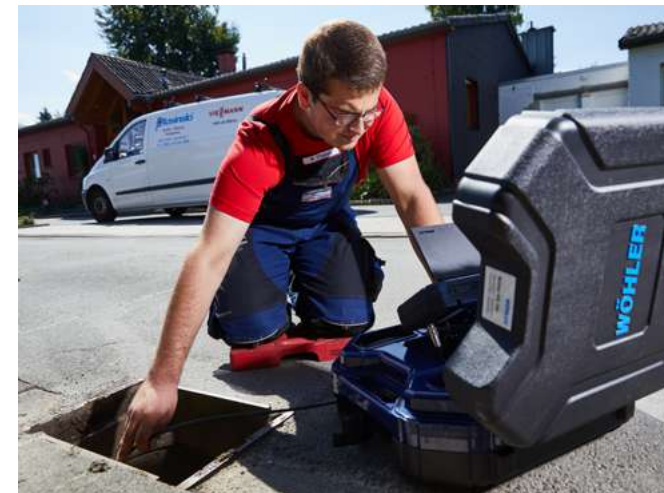
Secure drain inspection with the waterproof camera head.
