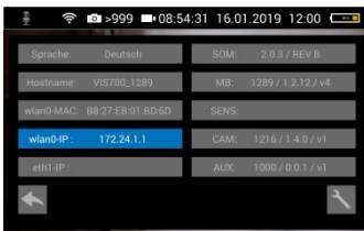
Fig. 55: Info-menu with the WLAN-Access-Point-mode activated.
