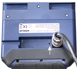
Fig. 61: Reset hole indicated by an arrow
