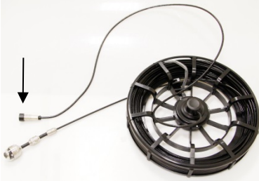
Fig. 68: Viper removed from the case, monitor plug covered by a lid
