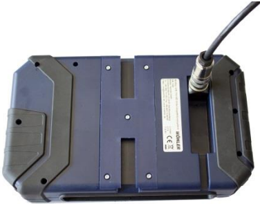
Fig. 10: Camera cable connection
