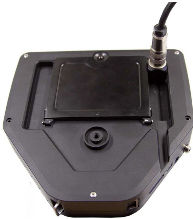
Fig. 8: Camera cable connection
