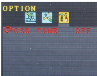
Fig. 19: automatic shutdown deactivated
