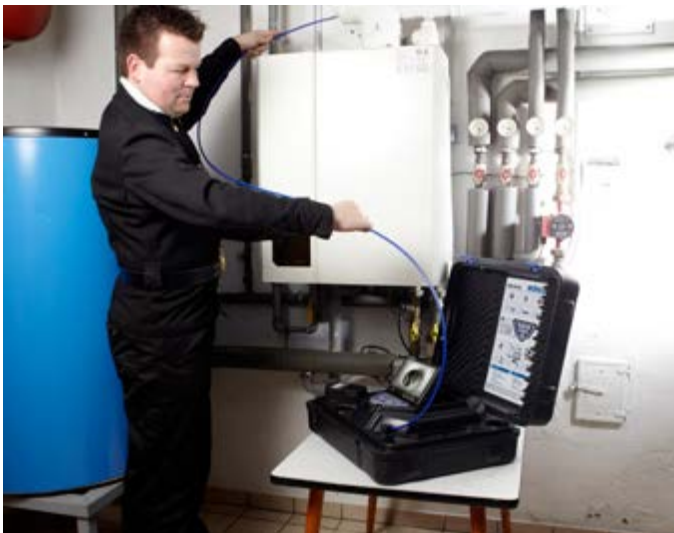
The 360° pan and 180° tiltable color camera head easily negotiates 87° bends.
