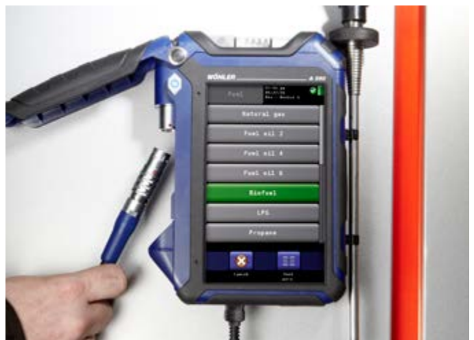
Convenient plug-in connection Analysis, temperature and draft – 3 functions in a single hose: Simply plug them together and fold down the protective lid.
