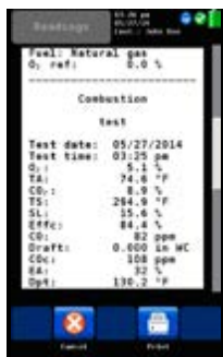
Print preview Generate a preview of the measurement before printing out the results.
