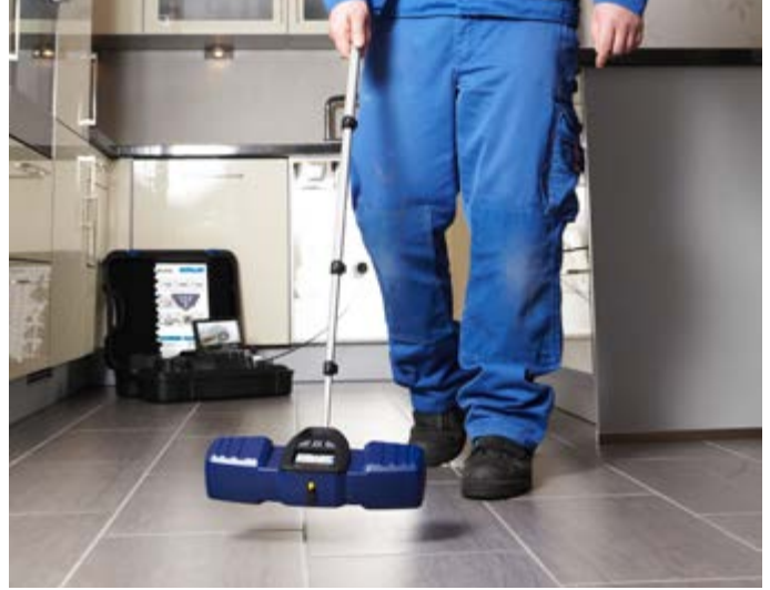
The actual distance count and the position of the head are displayed on the monitor. The Wohler L 200 Locator makes it possible to locate the camera head.
