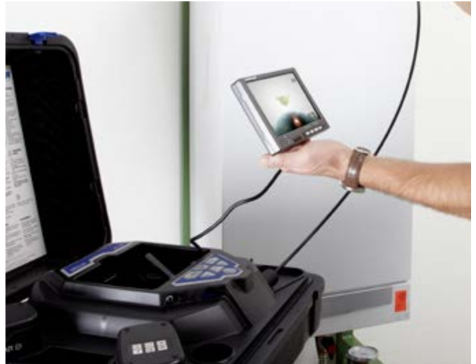
Tiltable and removable TFT wide-screen color monitor
