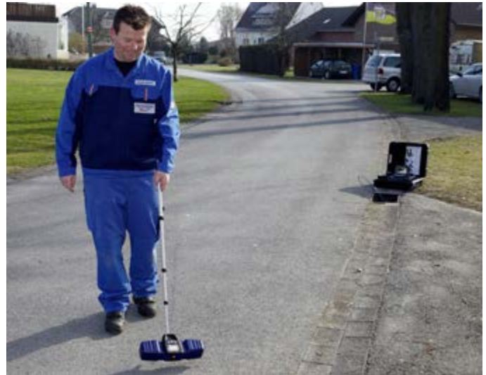
The Wohler VIS 350 precisely locates radio waves transmitted by the camera head through concrete and asphalt to save a lot of time and further building damage.
