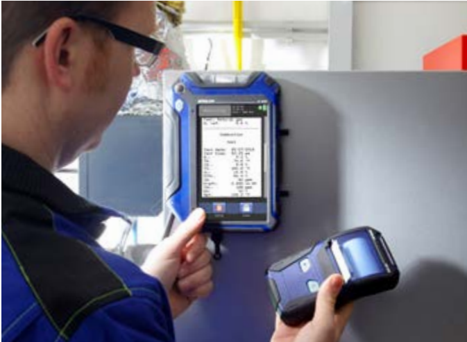
Printing out the results of measurements Printing out the results on the spot with the Wohler TD 100 Thermal Printer.
