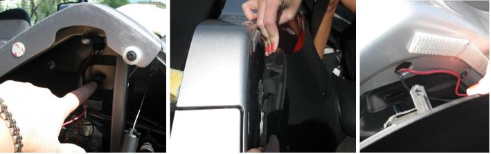
STEP 3: Unscrew the nut shown in the photo so that you can ground the black wire behind it. Once it is loose, place the circle ground clamp that you have attached to the black wire provided in the tackle bag over the post. Now tighten the nut securely back in place, making a good ground connection.
