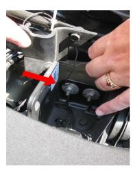
STEP 4: Locate the rubber grommet on the passenger side of the rear quarter panel in the trunk and unscrew it and the nut behind it.
