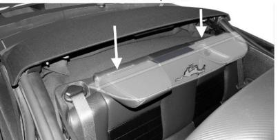
Step4- Keep the WindRestrictor® flat against the back of head rests. Rotate the head rests back into the fully upright position and make sure they lock into place. The WindRestrictor® will then be mechanically locked under the head rests. You are now finished with the install. If you have the illuminated version proceed to Step5.
