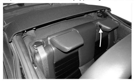
Step3- After you center the wind restrictor place it face down so that the locking tabs will slide between the head rests and the panel.
