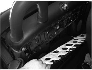
STEP 4- REMOVE THE CARPET BEZEL (B) IN TRUNK SURROUNDING THE THRUWAY AND OPEN THE LID. THIS WILL ALLOW YOU TO PULL BACK THE CARPET JUST A BIT TO GRAB THE WIRE WHEN RAN FROM CABIN.
