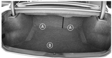
2. REMOVE ALL RIVETS THAT HOLD CARPET PANELS IN PLACE IN REAR AND ON PASSENGER SIDE BY TAIL LIGHT. THE ONE WITH A LOOP THAT YOU PULL REQUIRES A LOT OF FORCE. ROCK IT BACK AND FOURTH WHILE PULLING HARD.
