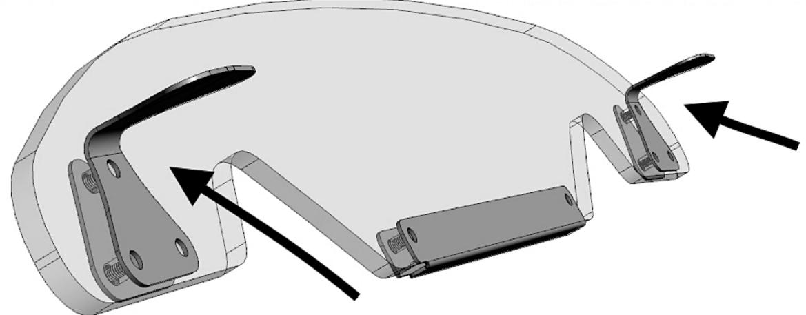
Step-2 Align and center the deflector on vehicle prior to removing protective covering of the bracket tape. Mark the outside edge of brackets with painter's tape to use as a guide once product is centered. Remove covering from bracket tape.
