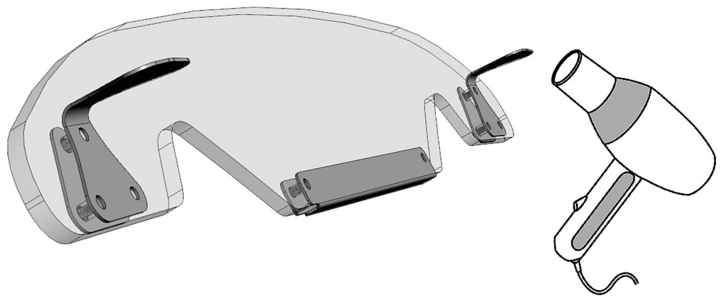
Step-4 Center the product between the painter's tape on panel. The two screws on bar (A) should perfectly line up with the two indentions on the tonneau cover (B). After confirming product is centered apply <a href="FIRM">FIRM</a> pressure simultaneously to front and top side of bracket for 20 seconds. If you have the illuminated version proceed to step 5. If you do not have the lighted version you are now finished!
