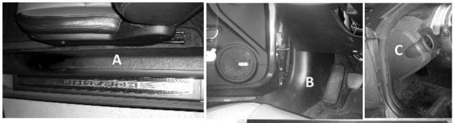
5. Remove trim panels marked A, B, C in these photos. (A) should be removed first. The panels are held in place by some push clips so just pull them away from the mounting surface and they should come unclipped with enough force. The grounding nut we've located is behind panel C. The harness with wiring is behind panel B.
