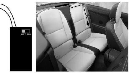
For best results, the unit should be used with your windows in the up position. The Windrestrictor will only block the rear wind gusts for the passangers, not the side windflow.
