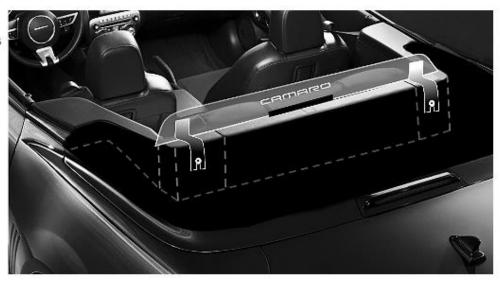
4. Hook the wires up from the Windrestrictor to the battery pack and install a new 9V battery. The wire from the light bar can be ran directly behind the seats and along side the passanger seat, mounted with velcro to the side panel.
