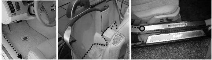
2. Clean the carpet retainer panel with the alcohol pads provided. Please insure that there is a clean, dirt and dust free surface. Do NOT use any oil based cleaners such as Armor All. Allow surface to dry. Peel the adhesive covers off of the bottom of the new door sills. It may help to fit on the sills with the covers still in place so that you can see how they are supposed to fit before installing them. Make sure you have tested your lights before this step. \*\*\*
