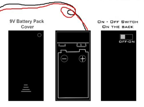
To utilize your battery pack simply connect the red wire from pack to red wire from LED lighting strip then do the same with black wire. Make sure the wires are taped up so that they do not touch each other. Put battery in the holder and turn switch to the "ON" position. You should see illumination at night.
