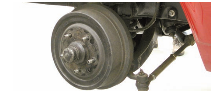
Using a breaker bar and the correct size socket, the wheels were removed from the car. If you want to speed things up you can use an impact gun.
