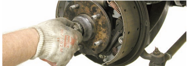
After the cotter key was removed, the spindle nut and large flat washer were disconnected with a large Crescent wrench and then the nut was loosened by hand. After the nut was disconnected, the hub assembly was removed. The nut and washer were retained for use later.
