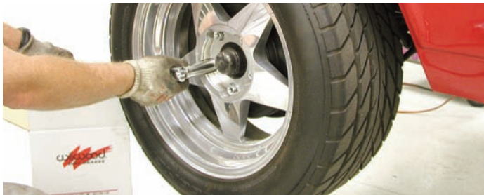
Using a breaker bar and the correct size socket, the wheels were removed from the car. If you want to speed things up you can use an impact gun.
