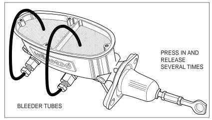
Typical Bleeder Tube Setup and Use
