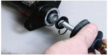
After the snap ring was disconnected from the unit, the pushrod, the snap ring and the washer were removed from the assembly.
