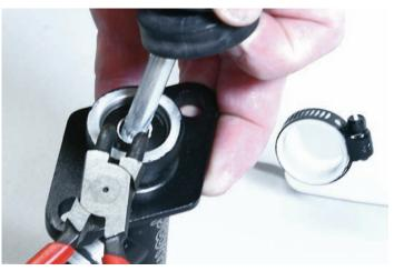
The rubber boot was disconnected from the back of the master cylinder far enough to access the snap ring that holds the piston inside of the bore.
