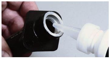
A few drops of Wilwood lubricant was placed inside of the piston bore and then it was distributed evenly inside of the bore. This can be done with finger power.
