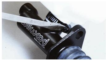
Using a flat blade screwdriver, the hose clamp connection was tightened to insure a good seal.
