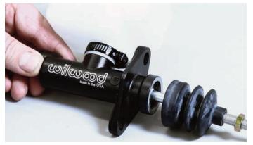
The rubber boot has to be connected to the master cylinder body and the plastic reservoir was installed on the top of the unit making sure the O-ring was used.
