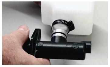
The hose clamp connection was loosened with a screwdriver and then the plastic reservoir was carefully removed from the master cylinder. Notice the O-ring seal that keeps this connection leak free.
