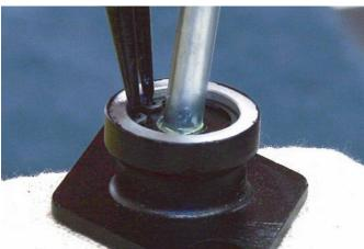
The pushrod was installed into the piston far enough make room for the snap ring to be installed. It is important for the snap ring to sit inside of the groove.
