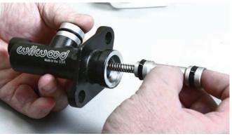
The piston assembly was carefully installed back into the master cylinder bore making sure it slides in easily.
