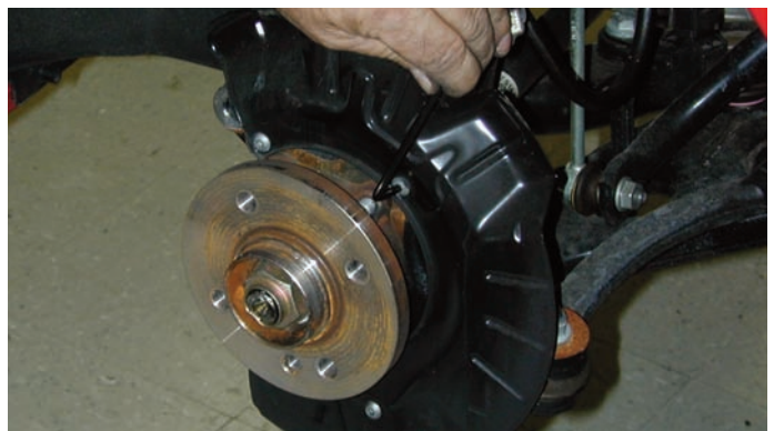
Using an Allen wrench, the bolts that secure the dust shield to the spindle were disconnected and then the dust shield was removed.
