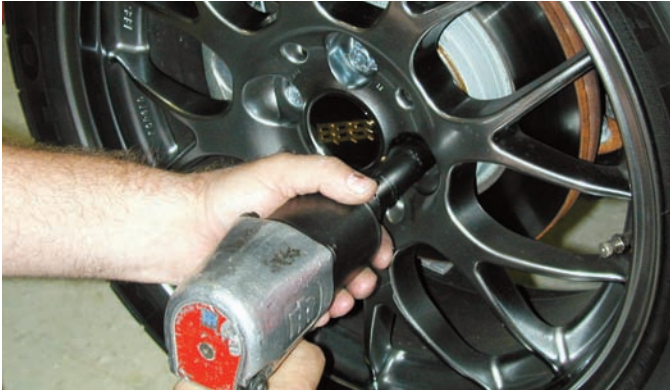
The car was elevated using a floor jack and then jack stands were placed under the car for safety. Using an impact gun and the correct size socket, the lug nuts were disconnected and the wheels and tires were removed.
