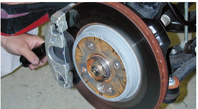
Using a long socket wrench and the appropriate size socket, the two bolts that secure the caliper to the bracket were removed.
