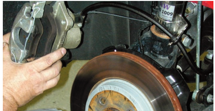
After the mounting bolts were disconnected, the caliper was lifted off of the spindle and rotor.
