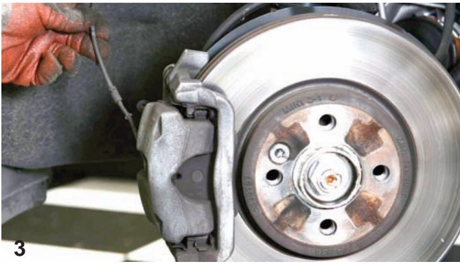
3 The original flexible brake line was disconnected from the steel hard line in preparation of removing the caliper. There is a rubber grommet on each flex line so it was removed and retained for reinstallation on the new Wilwood Flexline.
