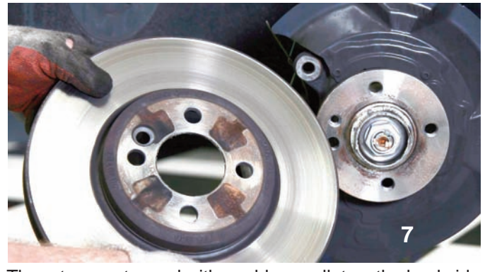
7 The rotor was tapped with a rubber mallet on the backside to break it loose from the hub assembly. When it was loose, it was removed from the assembly.
