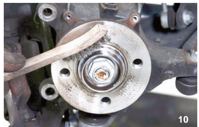
10 Before going any further, a wire brush was used to clean the grease and grime away from the hat locator on the hub.
