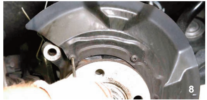
8 Using a torx screwdriver, the small screws that fasten the dust shield to the hub assembly were removed.
