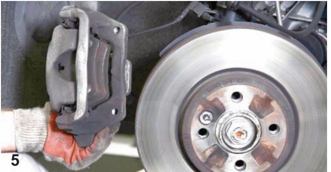
5 After the bolts were disconnected, the cast iron caliper was removed from the brake assembly. The new brake caliper is much lighter than the old caliper.
