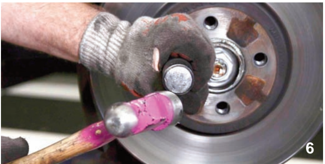
6 The torx bolt that secures the rotor to the hub was very tight, so it was loosened with an impact screwdriver. The bolts were retained because they will be used to fasten the new rotors.
