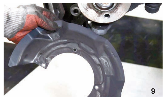
9 The dust shields were discarded because they will not be used with the new brakes.
