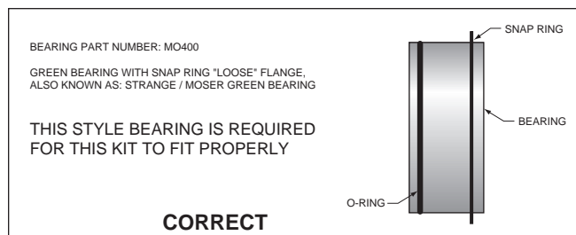
Figure 2. Loose Fit Bearing Configuration
