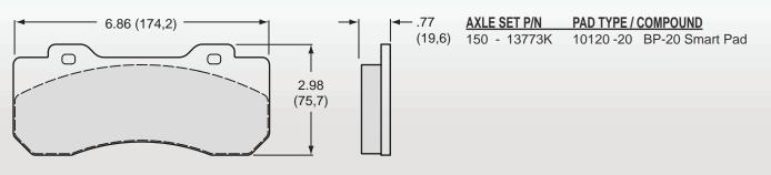
TX6R Caliper, Type 10120 Brake Pad Dimensions and Ordering Information
