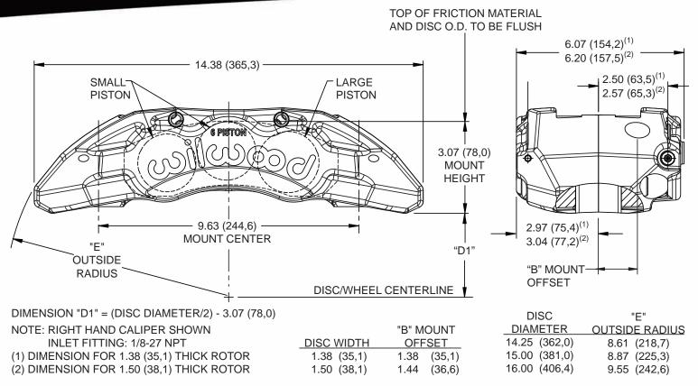
**TX6R Caliper, Dimensional Characteristics**
