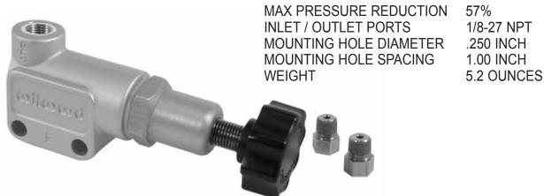
**INSTALLATION & ADJUSTMENTS** - Proportioning valves are normally installed in the rear fluid line to prevent the rear wheels from locking before the front wheels, or to give a driver the ability to make fine adjustments in front to rear bias percentage on the track to compensate for tire wear, fuel load burn-off, or changing track conditions. It is generally not recommended to attempt to reduce front wheel braking capacity.
