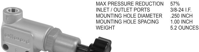
**INSTALLATION & ADJUSTMENTS** - Proportioning valves are normally installed in the rear fluid line to prevent the rear wheels from locking before the front wheels, or to give a driver the ability to make fine adjustments in front to rear bias percentage on the track to compensate for tire wear, fuel load burn-off, or changing track conditions. It is generally not recommended to attempt to reduce front wheel braking capacity.
