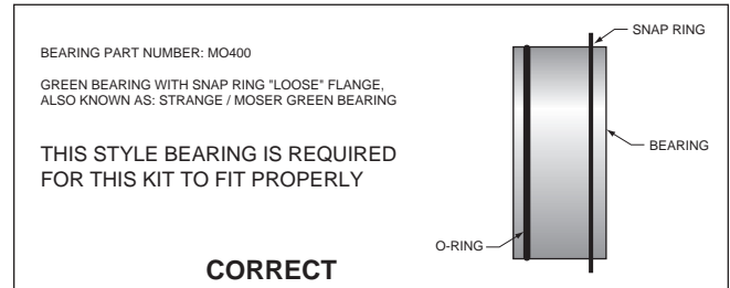
Figure 2. Loose Fit Bearing Configuration
