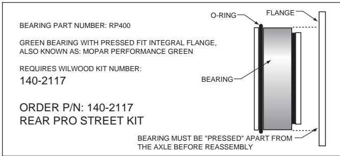
Figure 1. Press Fit Flange Bearing Configuration
