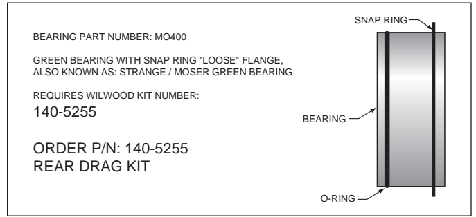
Figure 2. Loose Fit Bearing Configuration
