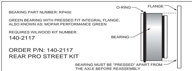
Figure 1. Press Fit Flange Bearing Configuration
