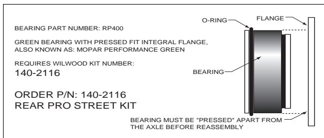
Figure 1. Press Fit Flange Bearing Configuration
