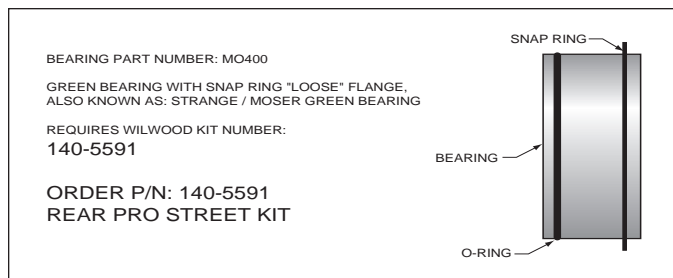
Figure 2. Loose Fit Flange Bearing Configuration
