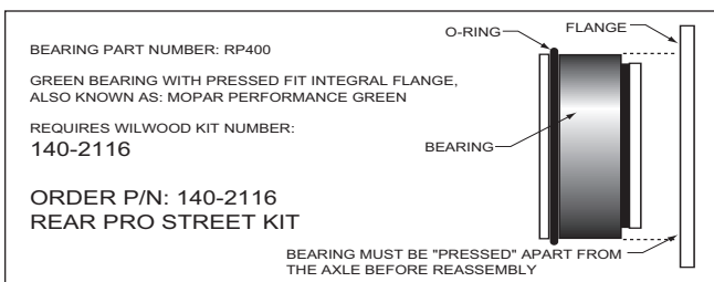
Figure 1. Press Fit Flange Bearing Configuration
