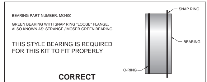
Figure 2. Loose Fit Bearing Configuration
