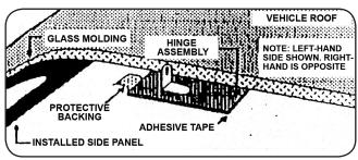
Place the louver on the window with the leading edge of the top slat as close to the window molding as possible and centered side to side. Using a soft lead pencil, mark lightly on the molding the location of the two hinge holes at the top of the louver. Then mark the location of the two tie down stude at the lower outside edges. When all four marks have been made on the molding, take the louver off the window. (On cars without edge molding on the glass, use a crayon and mark the glass-itself).
