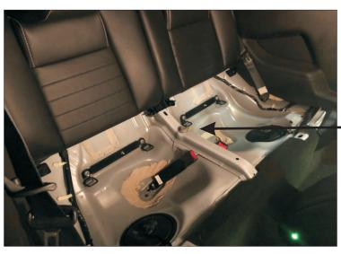
• Loosen and remove 1x 24mm mounting bolt (don't discard).
