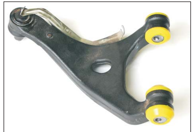
Fig 2 - left control arm with new bushes.
