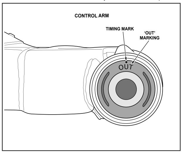
Press bush into eye with timing mark toward top of arm and 'OUT' marking facing away from centre of arm as shown.
