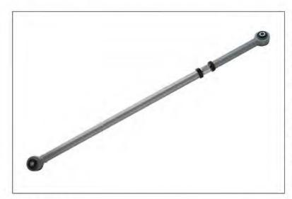
KPR068 - REAR PANHARD ROD (on-car adjustable) Adjustable rear Panhard Rod for the S197 chassis Mustang replaces factory bar to keep the rear axle located in optimal position. Features an on-car adjustable turnbuckle design ideal for street and track use. Improves rear handling characteristic and improves traction.
