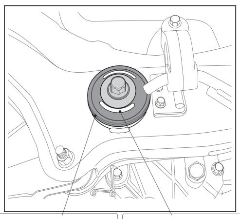
Bush removal is best achieved with the use of an air hacksaw. Cut down through the rubber voiding and steel shell being carefull not to damage the subframe housing.
