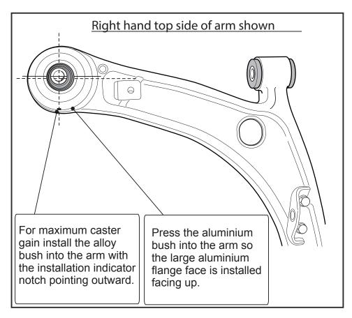
Remove the arm from the vehicle and press the oe bush out of the arm.
