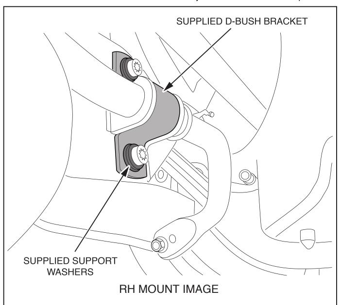
NOTE: Caution must be taken when installing the BWR21XZ 24mm rear sway bar to the vehicle without fitting the front BWF19 series or BWF20 series front swaybars as the balance of the vehicle will be altered. This may cause the vehicle to oversteer during sudden braking/steering manoeuvers.
