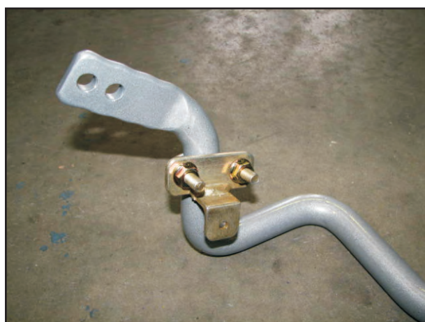
Photo 2. Whiteline Swaybar ride height sensor mounting bracket
