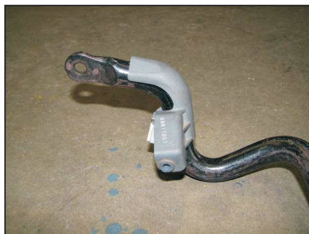
Photo 1. OEM Swaybar ride height sensor mounting bracket
