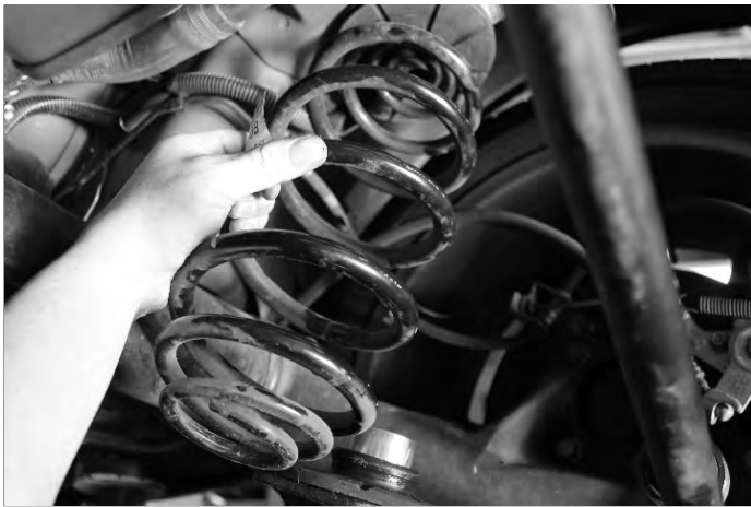
Re fit spring pads and coils
