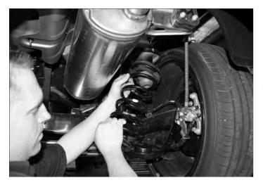
• Once the lower shock mount is unbolted, slowly raise the body - careful to not stretch the brake lines.
