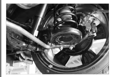
• Once hardware is tight, re-fit coils and lower shock mount.
