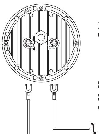
This product may be used with either 12 or 24 volt systems. Additionally, it is not polarity sensitive.
