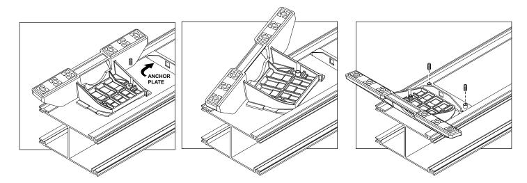
NOTE: Model MKAJ is an adjustable mounting foot. On this model you may loosen the screws on the rear of the foot and adjust the angle of the lightbar. To be used if the angle of the roof is not level with the road.
