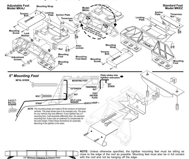
**IMPORTANT:** For strap mounted bars, be sure you have the right sized lightbar for your vehicle. The lightbar should be about the same width as the vehicle roof. If the lightbar is too large or small it will not mount properly to the vehicle and may shift or come loose during driving.
