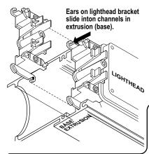
Lighthead mounting holes snap into the raised bosses on the lighthead bracket.
