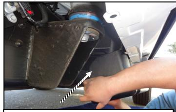
Remove the plastic cover by pulling it toward the side of the truck.
