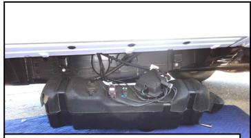
Carefully bring the tank down trying not to tilt or twist the tank to avoid damage to connectors.
