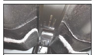
Using a ratchet with a long extension and a 13mm socket to loosen and remove the bolts of the tank support straps. Use an assistant to help hold the tank.
