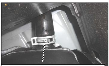
Use a set of pliers to loosen the hose clamp that is under the tank near the front of the truck that holds the filler hose. Carefully remove the filler hose from the tank.
