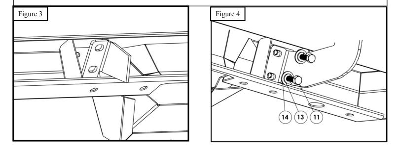
8. Below are Figures representing the orientation and positioning of the brackets for Crew Cab and Ext. Cab trucks.
