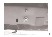
STEP 4: Remove the five factory nuts holding the brackets for the air conditioning lines.
