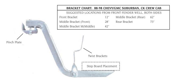
**STEP 3:** Attach the pinch plate portion of the brackets to the truck at the cab rail and tighten the 5/16" x 2¼" Hex Head Bolts and 5/16" Nylocks. Note: All the brackets should be loosely hanging from the truck.
