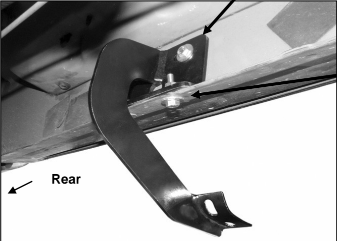
(Fig 3) Driver side-rear Mounting Bracket location
