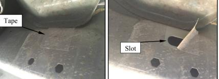
2. Place Stud/nut plate onto the slotted hole (Item 7) as well as the hex riv-cert (Item 8) onto the hexagon hole. (Before inserting stud/nut plate onto the slot place a square plastic retainer (Item 23) on the stud portion of the plate to prevent the plate from falling in the slot, as shown in picture below).
