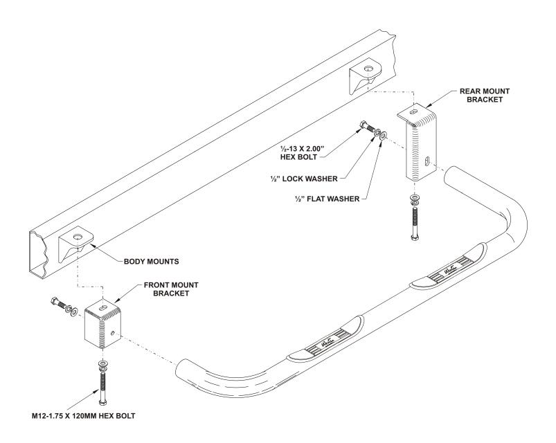
ASSEMBLY AND INSTALLATION VIEW OF DRIVER SIDE - PASSENGER SIDE OPPOSITE
